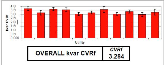
Effect of CVR on kVAR is more significant than on kW
